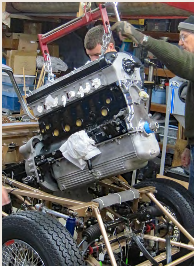
The engine goes in at a steep angle due to the transmission having to be attached to it. This required an engine hoist with a leveler for best results. The engine was lowered in gradual increments and a dolly put under the back of the transmission to help steady it.
