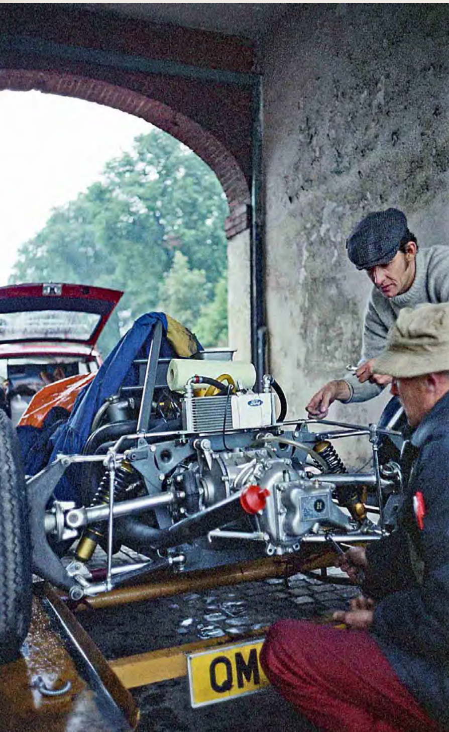
Myself and Roy sheltered from the rain at Oulton Park. Debris in the clutch prevented any engagement. Fortunately we were able to flush everything out.
