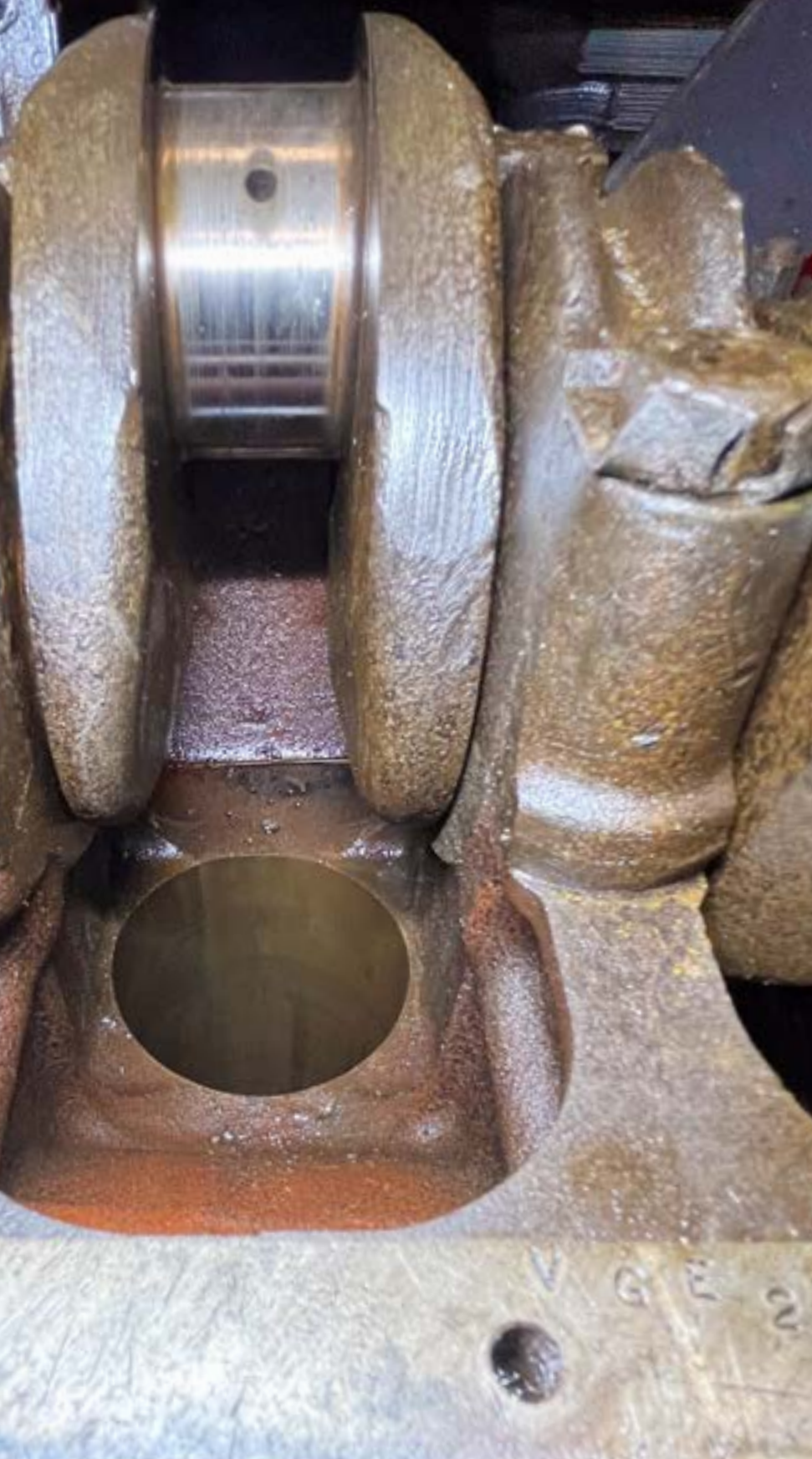
Most cathedrals have less structure than this stout boxed bottom end of the XK engine.
